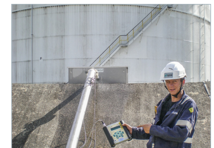
For Antoine Henri and his colleagues from Flexim France, setting up a temporary flow measurement point in next to no time with the portable FLUXUS® F601 is an everyday routine task.
