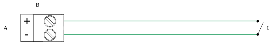
Figure 3-20: Discrete input Input Wiring (Internally Powered)
