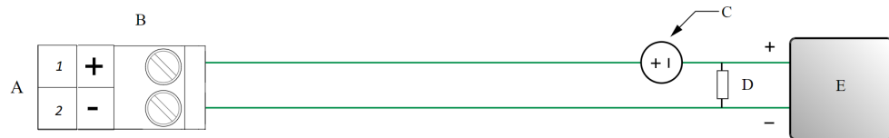
Figure 3-13: Frequency output wiring (externally powered)
