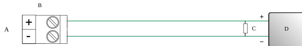
Figure 3-17: Discrete output wiring (internally powered)
