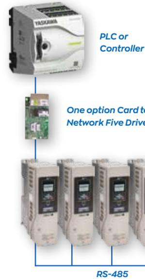
Reduce the number of option cards up to 80%. Only a single communication option card is required to network up to five drives via the RS-485 terminals.
