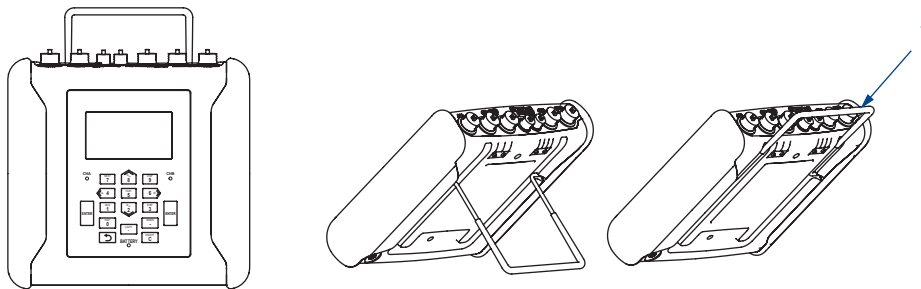
Fig. 6.3: Hanging up the transmitter
